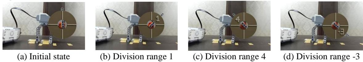
Figure 15: Example of VtoR's Rotation
