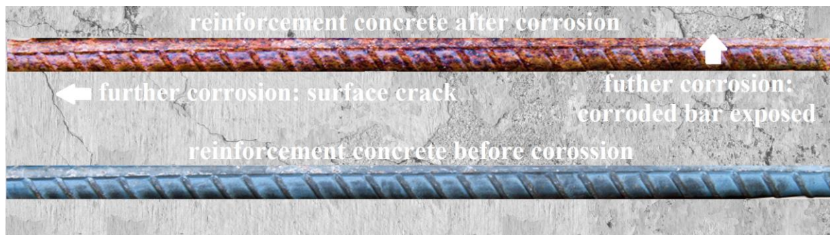
Figure 1: Example of influence reinforcement concrete after corrosion
