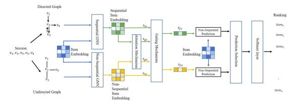
**Figure 1:** Overview of SR-DGN model. For each session *s*, directed and undirected graphs are constructed and sequential and non-sequential item representations are learned using sequential and non-sequential GNN models respectively. Using shared learnable parameters, the final sequential and non-sequential session representation is learned. Finally, the best prediction is selected for making recommendations.
