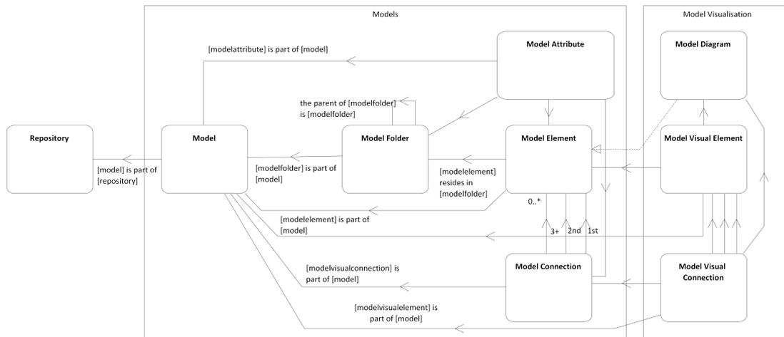
**Figure 7:** Model storage structure
