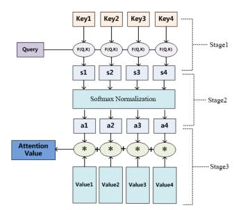
Figure 4 Attention mechanism calculation process
