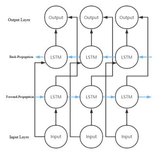
Figure 3 Bi-LSTM network structure diagram
