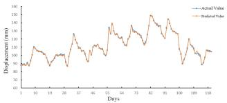
Figure 6 CNN-Attention-Bi-LSTM-Attention landslide prediction model result curve
