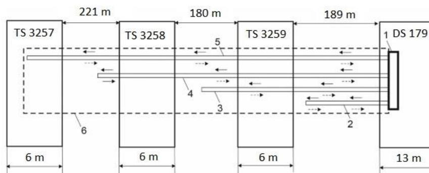
**Figure 2.** Conditional scheme of laying fiber-optic conductors
