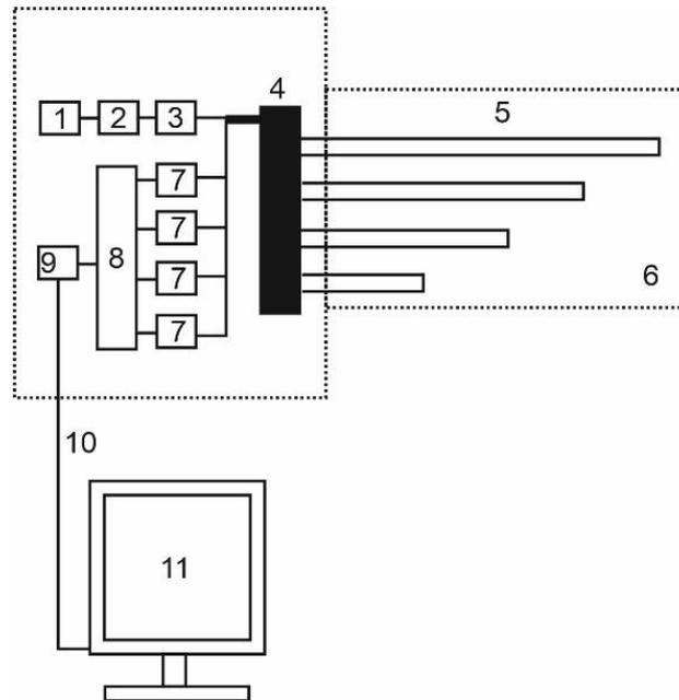
**Figure 10.** Structural diagram of the laboratory sample of the ACCS. Where 1 – laser power supply; 2 – semiconductor laser with a wavelength of 650 or 850 nm; 3 – optical polarizer with an insulator; 4 – optical coupler; optical fiber input and output device (cross); 5 – single-mode fiber-optic conductor (G652 sensor); 6 – cable channel; 7 – photodetector; 8 – data preprocessing device; 9 – matching device; 10 – connecting cable; 11 – a computer with software.
