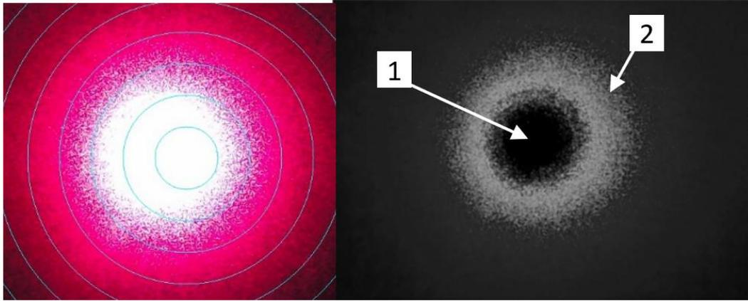
**Figure 8.** The shape of the light spot falling on the surface of the photo matrix. Where 1 – negative of the OF core; 2 – negative of the OF shell
