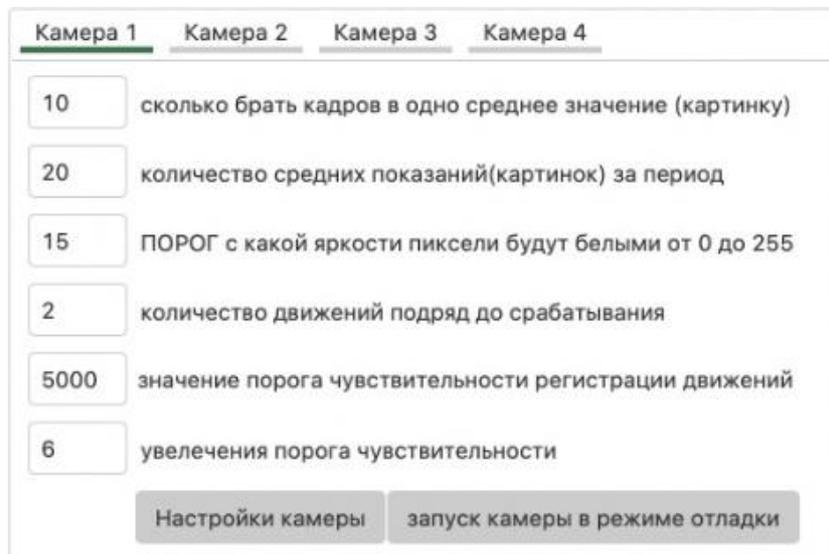
Figure 13. Camera setup block
