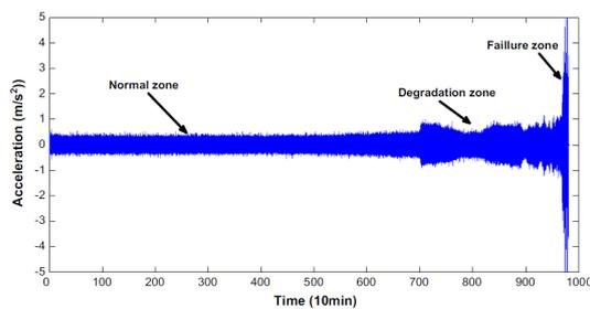
Figure 5: Bearing run-to-failure vibration signals[28]
