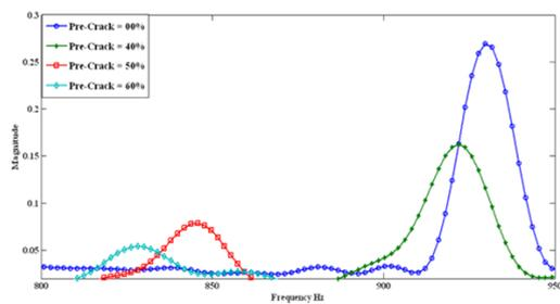
Figure 4: Vibration spectra for different cut depths at frequency range of 800 to 950 Hz[27]
