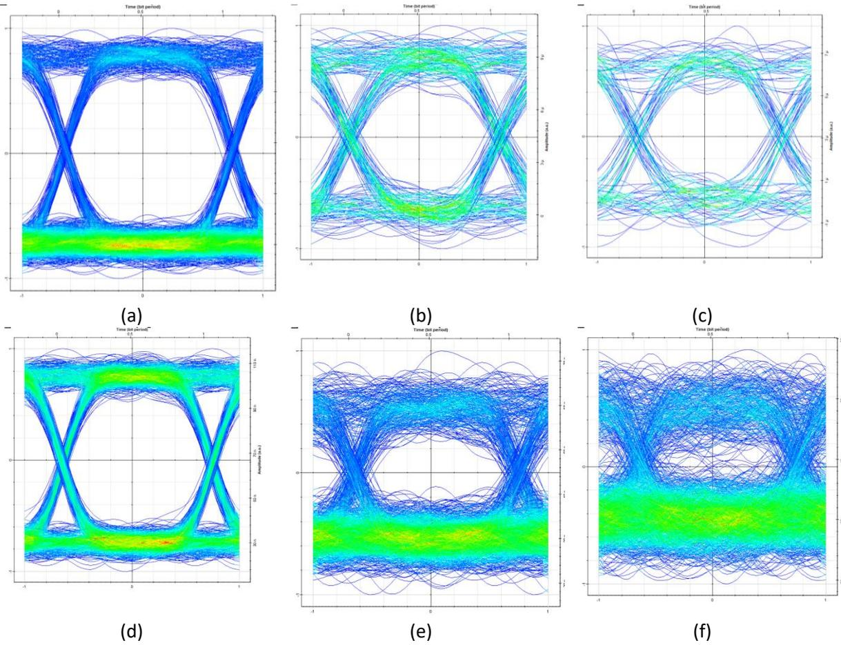
**Figure 3:** Eye patterns of the hybrid VLC-OCMA system using RD code over (a)70m, (b)60m and (c)50m VLC range for UP; (d)70m, (e)60m and (f)50m VLC range for DN transmission
