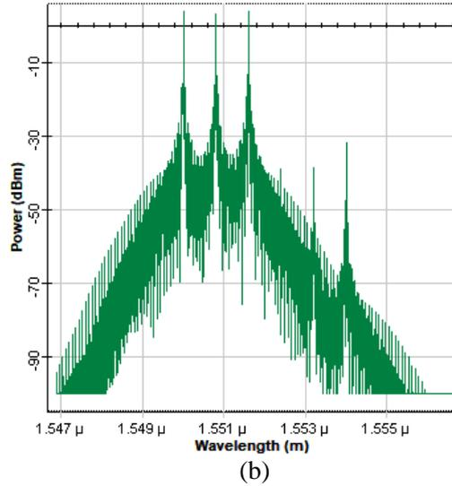
**Figure 6:** Measured spectra of the hybrid VLC-OCDMA system using RD code at (a) Tx and (b) Rx over 10m range at 10Gbps rate
