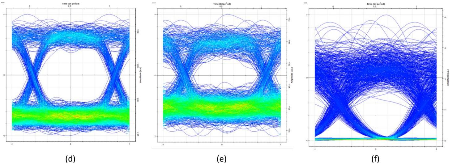
**Figure 4:** Eye patterns of the hybrid VLC-OCDMA system using RD code over (a)20Gbps, (b)60Gbps and (c)90Gbps VLC range for UP; (d)20Gbps, (e)60Gbps and (f)90Gbps VLC range for DN transmission
