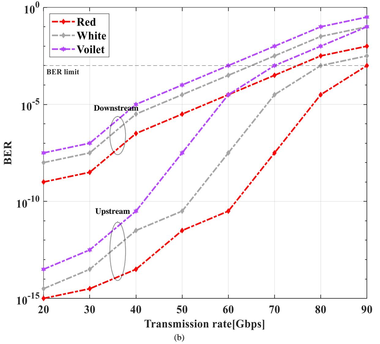
**Figure 2:** BER performance of proposed system for varied (a) VLC range employing different codes and (b) transmission rate for different LEDs using RD code
