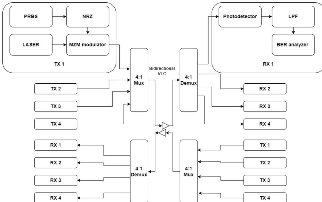
**Figure 1:** Block diagram of full-duplex hybrid VLC-OCDMA system
