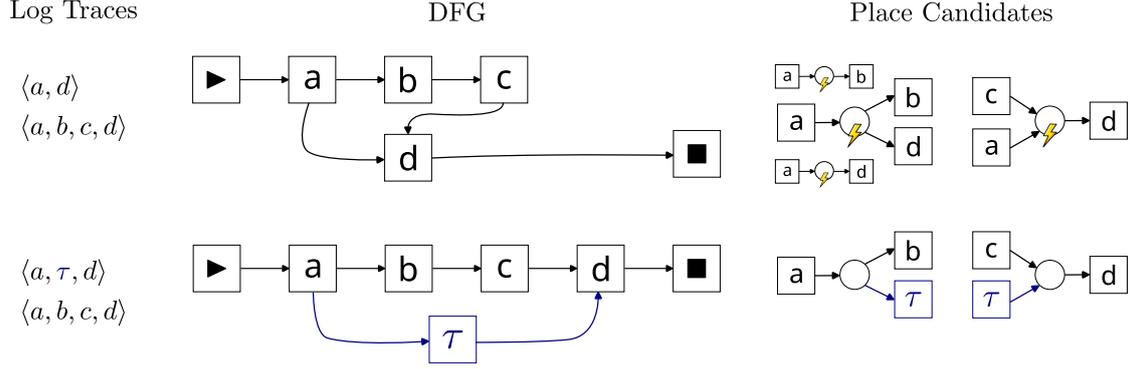
**Figure 2:** Two event logs and their DFGs showcasing the motivation for repairing implicit skips. The directly-follows relation between  $a$  and  $d$  would suggest considering place candidates with poor fitness. The second log, where an artificial activity  $\tau$  is inserted where  $b$  and  $c$  are skipped, mitigates this problem by replacing the directly-follows relation between  $a$  and  $d$ .
