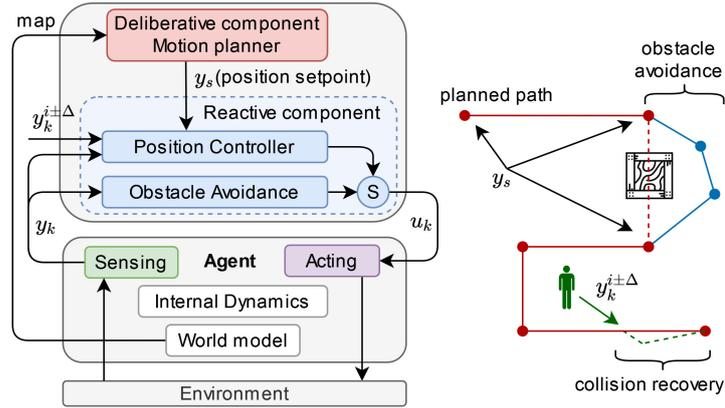
**Figure 1:** Deliberative-reactive control architecture for the pedestrian agent (left) and example (right).
