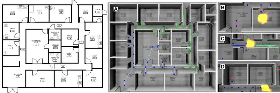
**Figure 2:** Floor plan [20] (left) and guidance indicators (right): A. visibility graph for fire drill case; B. office routes for fire in office; C. hallway routes for fire in hallway; D. office routes for fire in hallway.
