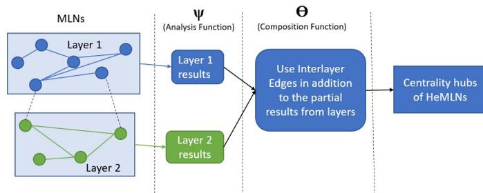
Figure 2: Decoupling Approach for HeMLN Degree Hubs
