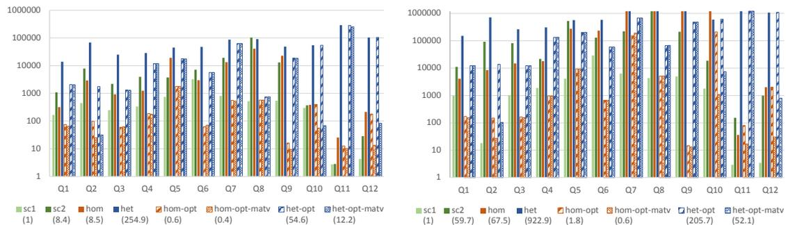
**Figure 4:** Evaluation times (ms) of queries  $Q_1\text{--}Q_{12}$  for scale factors 200K (left) and 2M (right). Numbers in parentheses are (geometric) mean evaluation times across queries normalized relative to *sc1* baseline (e.g., for scale factor 200K, query evaluation in *sc2* is 8.4 times slower than in *sc1*, on average).
