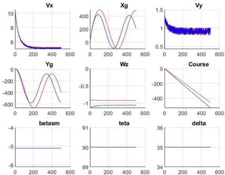
**Figure 4:** Graphs of changes over time of the single-screw vessel's movement parameters in turning circle: blue color – taking into account the rotation center displacement, red color – without taking into account the rotation center displacement
