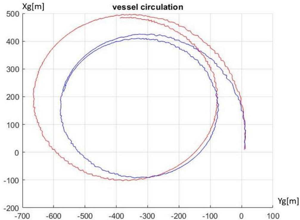
**Figure 5:** Turning circles of the conventional single-screw vessel: blue color – taking into account the rotation center displacement, red color – without taking into account the rotation center displacement
