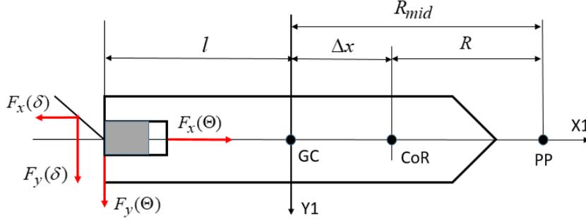
**Figure 2:** Control scheme of a conventional single-screw vessel
