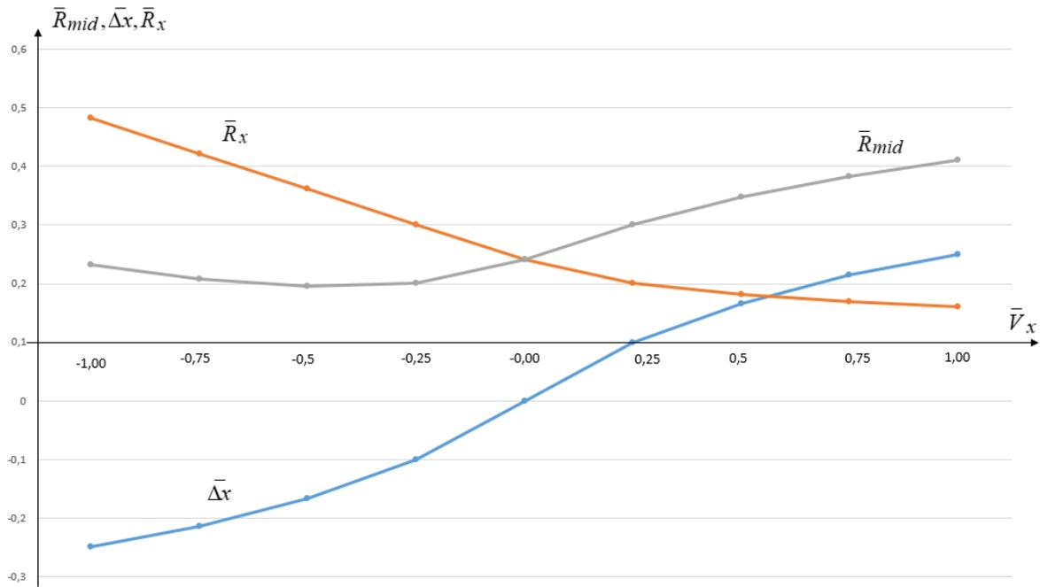
**Figure 3:** Dependence  $\bar{R}_{mid}, \bar{\Delta x}, \bar{R}_x$  on the reduced longitudinal speed of the vessel
