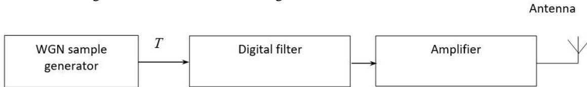
**Figure 7:** Block diagram of a noise generator
