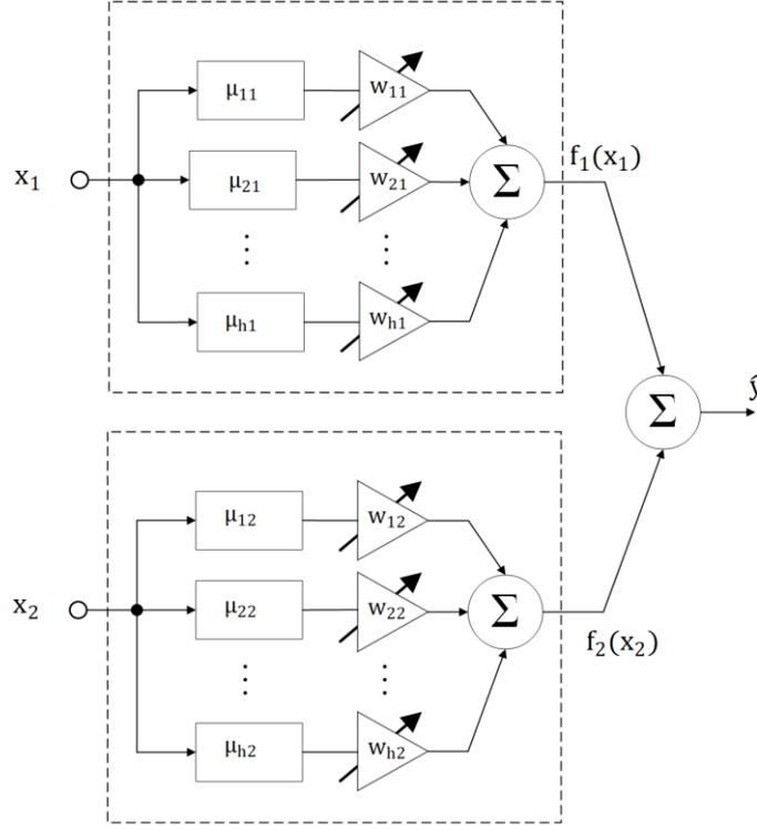
**Figure 2:** Architecture of neo-fuzzy neuron with two inputs
