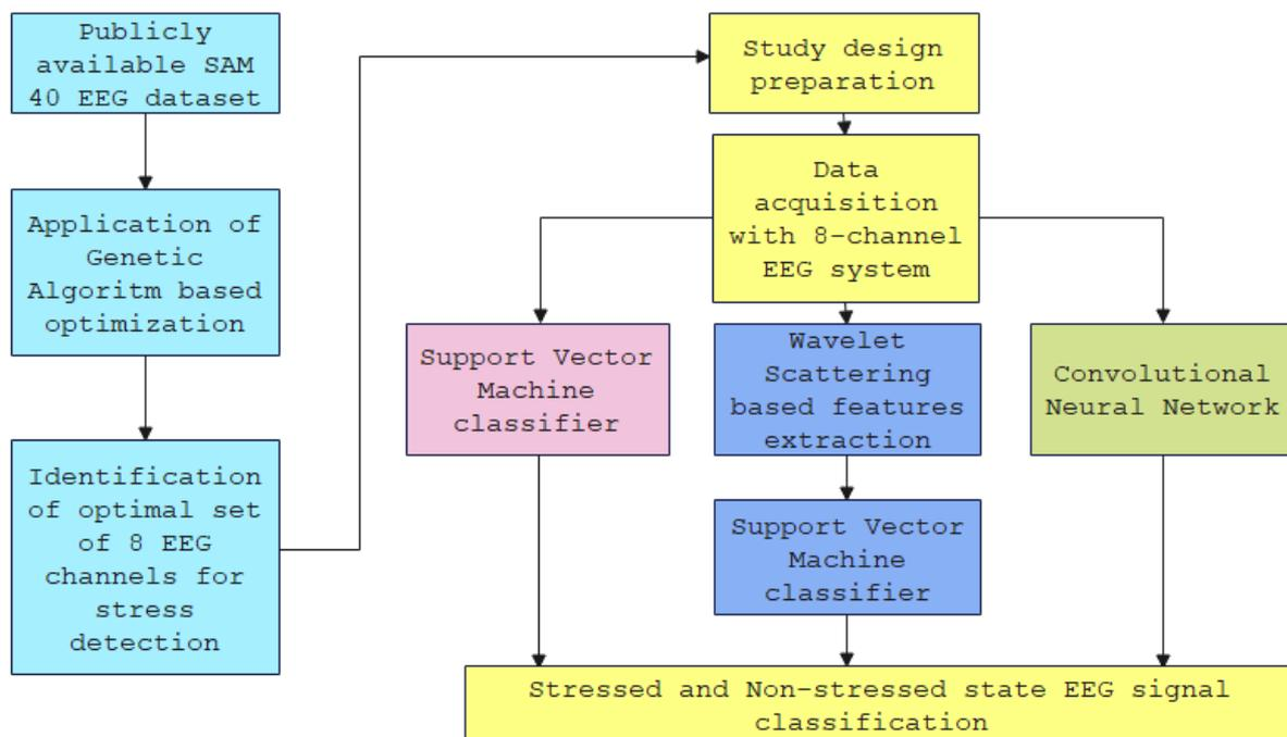
**Figure 1:** Block diagram depicting proposed methodology of using reduced channel EEG signal configuration for psychological stress detection
