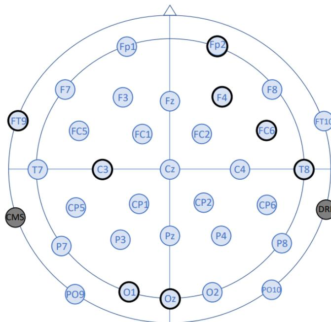
**Figure 3:** The 8 optimal EEG electrodes used for data acquisition in the study are highlighted
