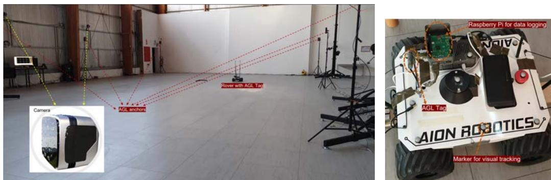
(a) Setup for benchmarking with motion capture system at ID2Move facility in Nivelles, Belgium. (b) Rover used in the motion capture benchmarking.
