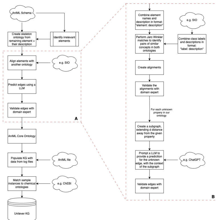
Figure 1: The AnIML2KG pipeline: the overall pipeline is shown on the left; Section A is expanded on the right (Section B) to illustrate the use of ontology alignment in the knowledge capture stage.
