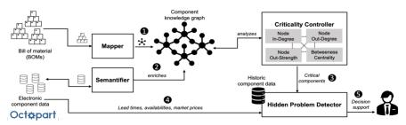
**Figure 5:** Model for graph-theoretic analysis of component criticality in supply chains: Hidden problem detector module.
