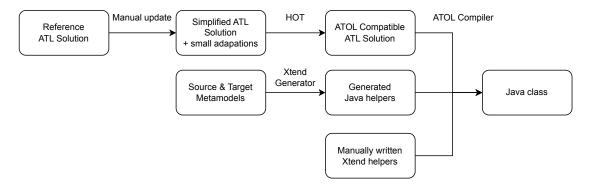
Figure 1: Compilation pipeline or the ATOL solution
