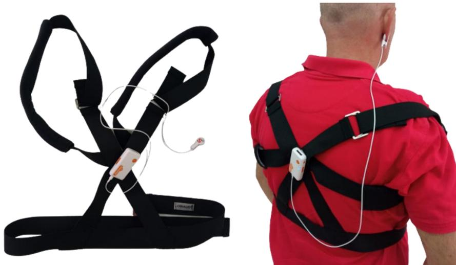
**Figure 1:** Placement of electronic device on the shoulder band (image on the left) and correct positioning of wearable sensor for acquisition of acceleration values and PPG signal (image on the right)
