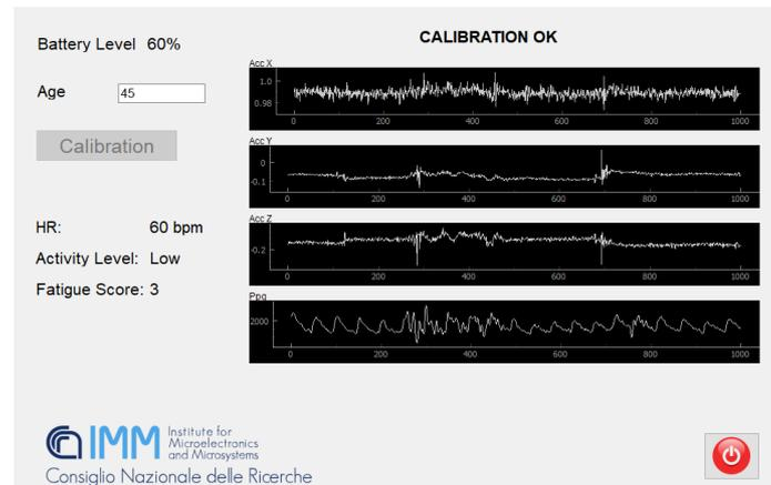
**Figure 3:** End user software interface. The right-hand side shows the data processed by the algorithmic pipeline (heart rate, activity level and fatigue score) while the central part plots the raw signals acquired from the wearable device used
