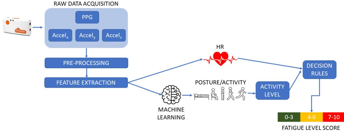
**Figure 2:** Proposed pipeline for fatigue estimation, through a logical block representation.
