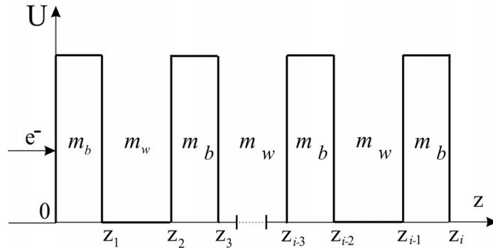
**Figure 1:** Schematic energy and geometric diagram of the studied multilayer nanosystem
