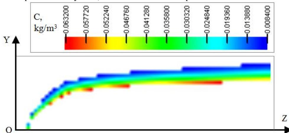
**Figure 11:** Mass concentration distribution of hydrogen within flammability boundaries in YOZ plane (wind speed makes up 1 m/sec)
