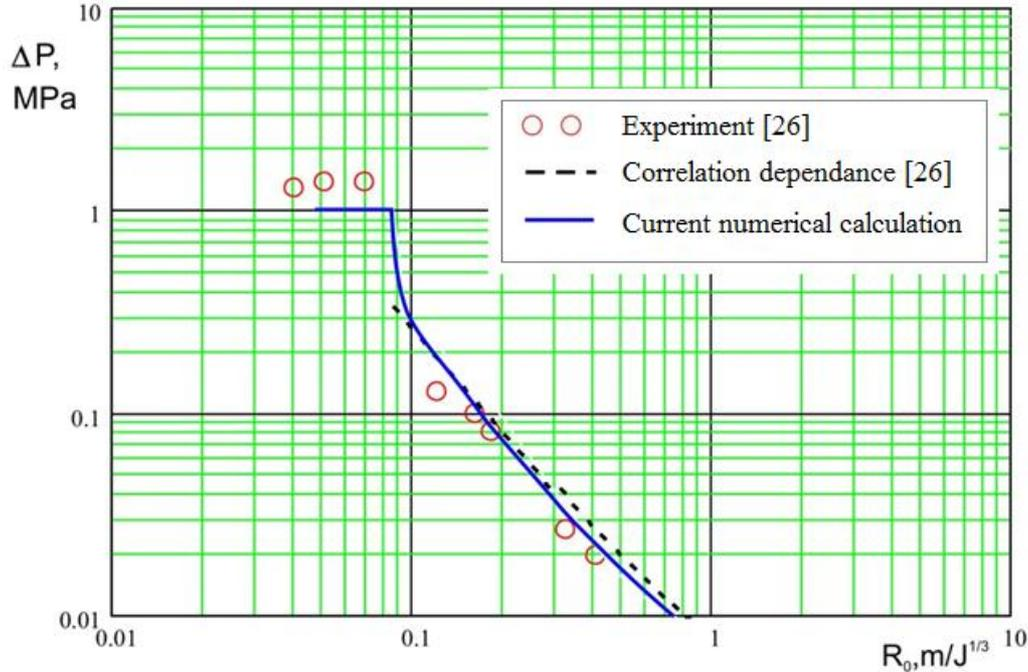
**Figure 5:** Explosion waves parameters in comparison with experimental data [26] and analytical correlation dependence [26]
