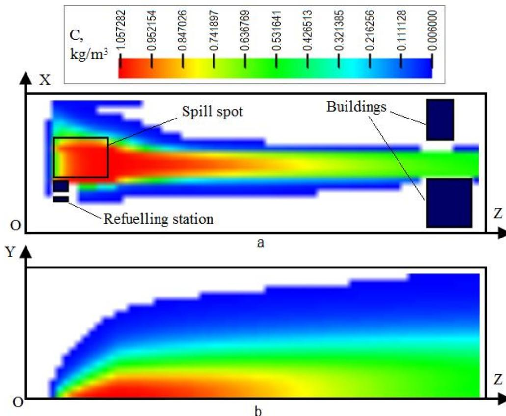
**Figure 6:** Numerical computations of spilled liquid hydrogen dispersion (wind speed 1 m/sec: a – the plane XOZ near the ground; b – the plane YOZ view)
