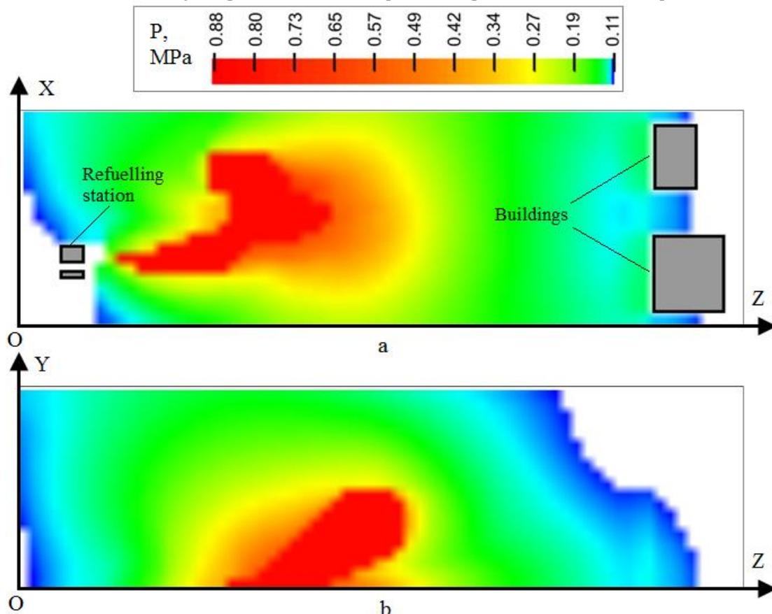
**Figure 12:** Pressure distribution after hydrogen explosion: a - near the ground; b - in YOZ plane
