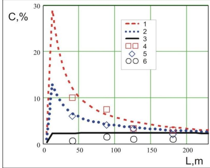
**Figure 4:** The maximal propane concentrations: 1, 2 and 3 – computations, 4, 5 and 6 – experimental data [25] at heights 0.8, 1.4 and 2.3 m, accordingly
