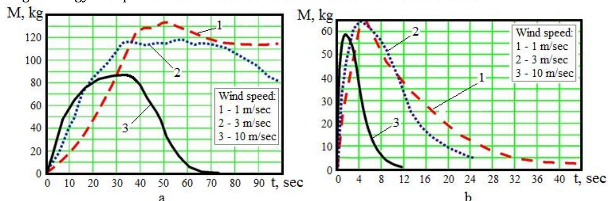
**Figure 10:** The history of total mass of gaseous hydrogen which mass concentration is within flammability limits (the air-hydrogen mixture could explode) during the dispersion process for different wind speed conditions : a – evaporation after spillage; b – after instant gas release
