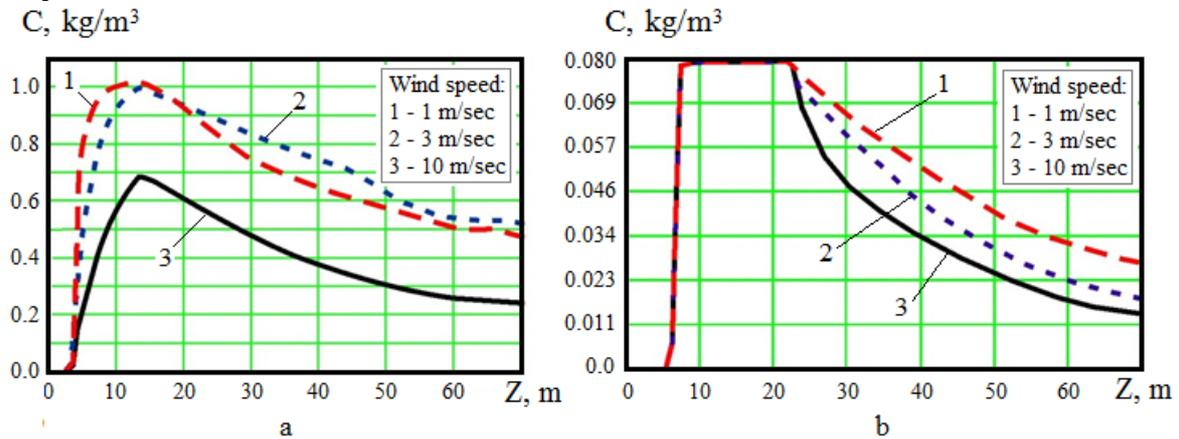
**Figure 7:** The maximum hydrogen concentration distribution along the OZ-direction for different wind speed conditions: a – evaporation from spill spot ; b – instant release of all the hydrogen amount
