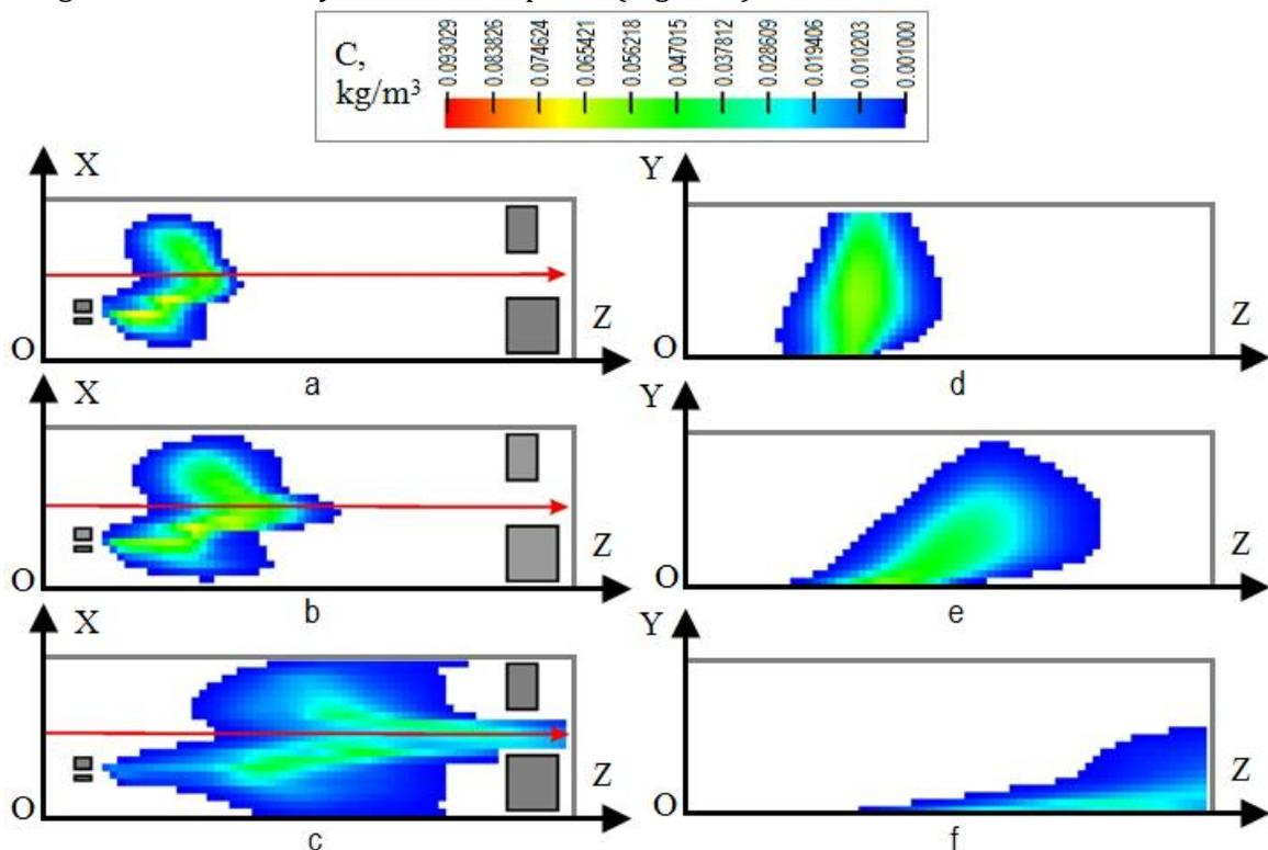
**Figure 8:** Hydrogen concentration distribution in 5 sec after release in planes XOZ and YOZ for different wind speed conditions: a, d – 1 m/sec; b, e – 3 m/sec; c, f – 10 m/sec
