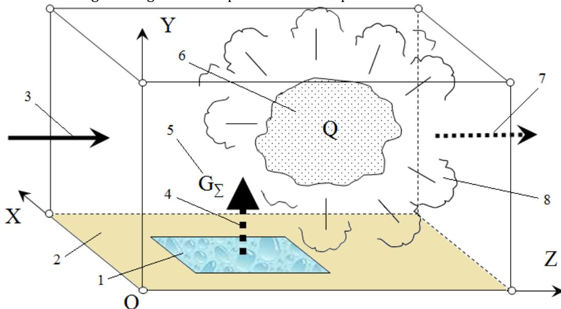
**Figure 3:** Calculation scheme: 1 – spill spot; 2 – ground surface; 3 – air wind vector; 4 – evaporation process; 5 – total evaporation rate; 6 – mixture; 7 – explosion products; 8 – overpressure explosion wave
