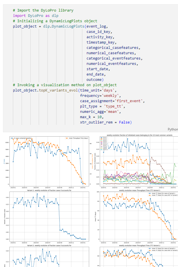
Figure 1: Example DyLoPro code: after having correctly initialized a DynamicLogPlots object, all of DyLoPro 's capabilities can easily be accessed by invoking the desired methods on the initialized object. All arguments used for initializing the object are assumed to be already specified. The invoked visualization method generates, i.a., for each of the 10 most frequently occurring variants, the weekly mean throughput time of cases pertaining to that particular variant, vs. cases pertaining to all other variants (and of which the first event occurred in that week).
