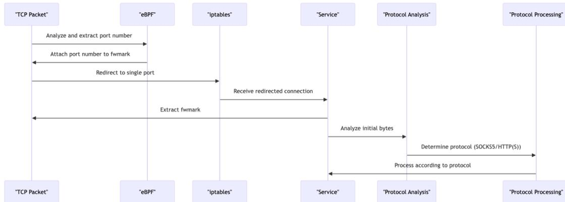
**Figure 8:** Sequence diagram illustrating the process of processing an incoming connection
