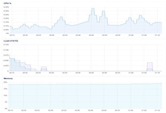
**Figure 12:** Demonstration of the Proxy Reactor load on VPS during idle time
