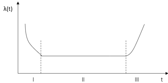
Figure 2: Area I—the period of running-in, Section II—period of normal operation, Area III—aging period
