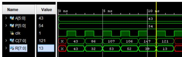
**Figure 5:** A time diagram of the operation of the modular number-squaring device with one-bit analysis of the RgA2 multiplier
