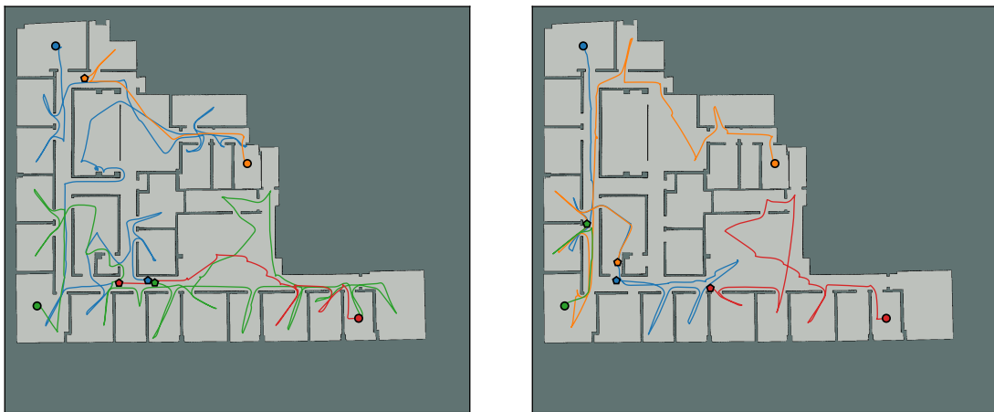
Figure 4: The paths followed by the robots using the classical frontier exploration strategy (FE, left) compared with our method (Ours, right). Each robot has a different color. The circles indicate the starting position of the robot, while the stars indicate the location when a robot joins a cluster. When robots are in the same cluster, we indicate only the trajectory of the leader. Each robot has its own map and its own SLAM module; we use the full map of the environment for visualization purposes.
