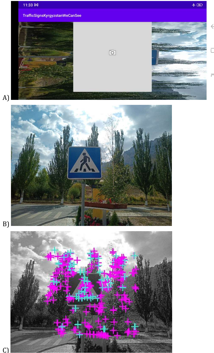
Figure 7: An example of the screenshot (A), an original image taken by the smartphone Doogee S96 Pro at cloudy weather (B), and a greyscale image with keypoints (C)
