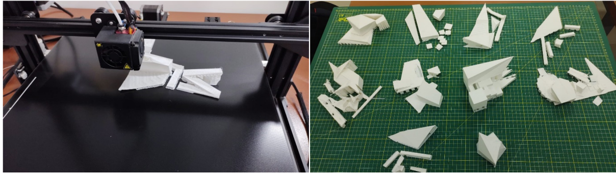
Figure 2: On the left, the 3D printing process. On the right the printed parts ready to be assembled.
