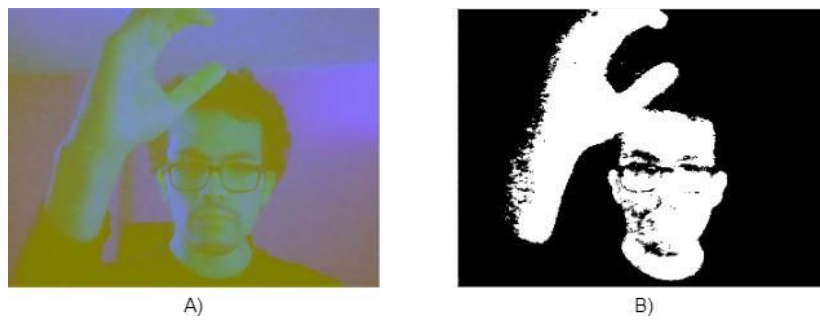
Figure 4: A) Frame with the YCbCr color model, B) Frame highlighting the sectors that have the skin color.
