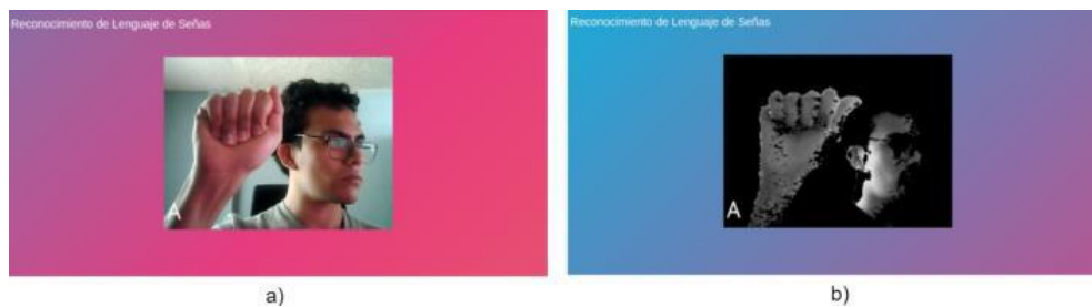
Figure 7: A) Execution of CNN model recognizing the static alphabet 'A' of the PSL on the web platform, visualized by the user, B) Preprocessing of the frame delivered to the CNN model for recognition of the static alphabet 'A' of the PSL on the web platform, not visualized by the user.
