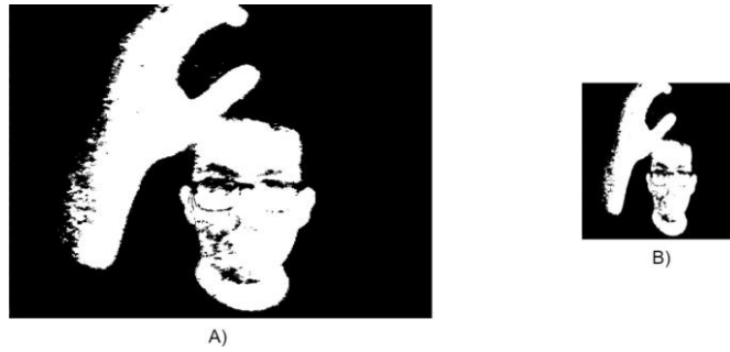
Figure 5: A) Frame with resolution of 640x480 pixels. B) Frame output with 224x224 pixels resolution change applied.
