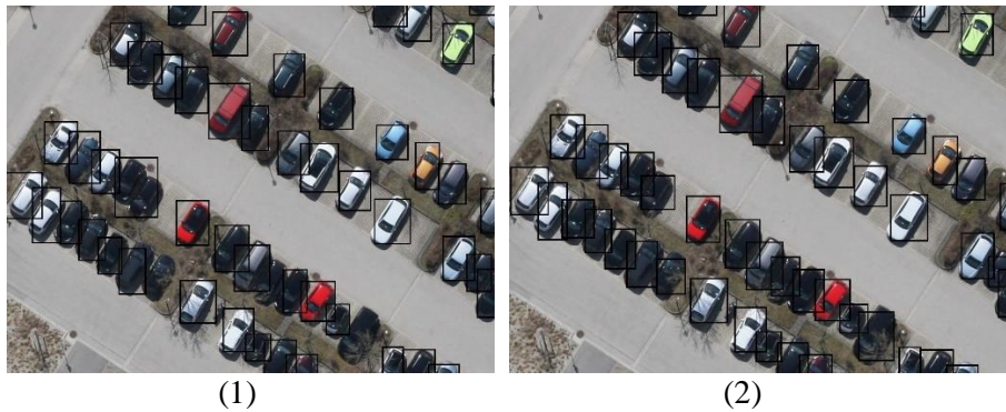
Figure. 5 . A comparative analysis of region boundary prediction for a network without a gap (1) and a network with a gap (2) shows differences in the quality of prediction. It is worth noting that the frames provided by the network with the connection of object map skips are significantly more accurate than those created by the network without connection (highlighted in yellow). Other parameters remain unchanged.
