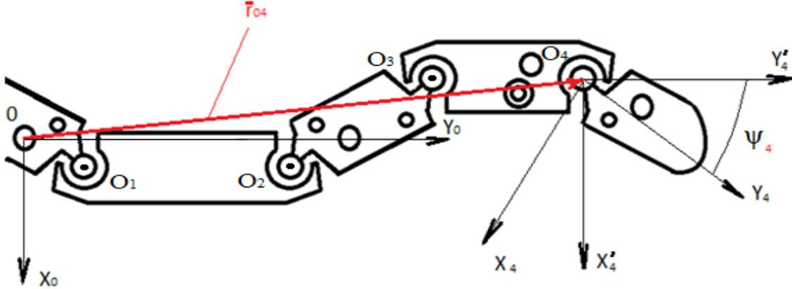
**Figure 4:** Kinematic diagram of articulations of the phalanges of one finger with elements of the palm of an anthropomorphic prosthesis
