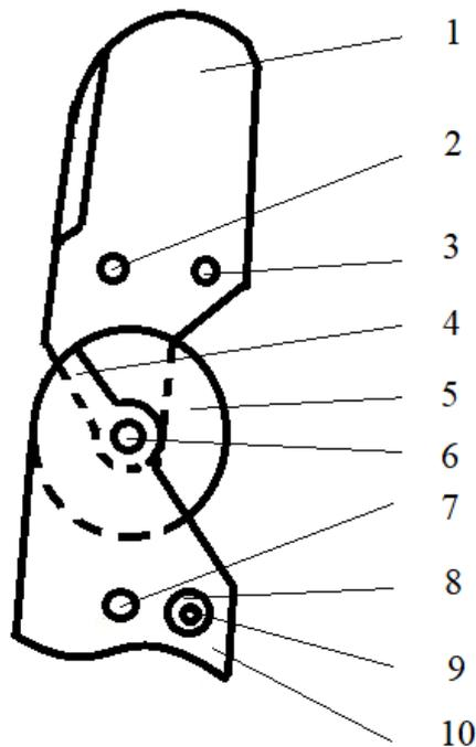
**Figure 1** : Schematic representation of the kinematic diagram of articulation of the phalanges of the prosthetic finger
