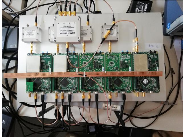
**Figure 3:** Photograph of the receiver platform
