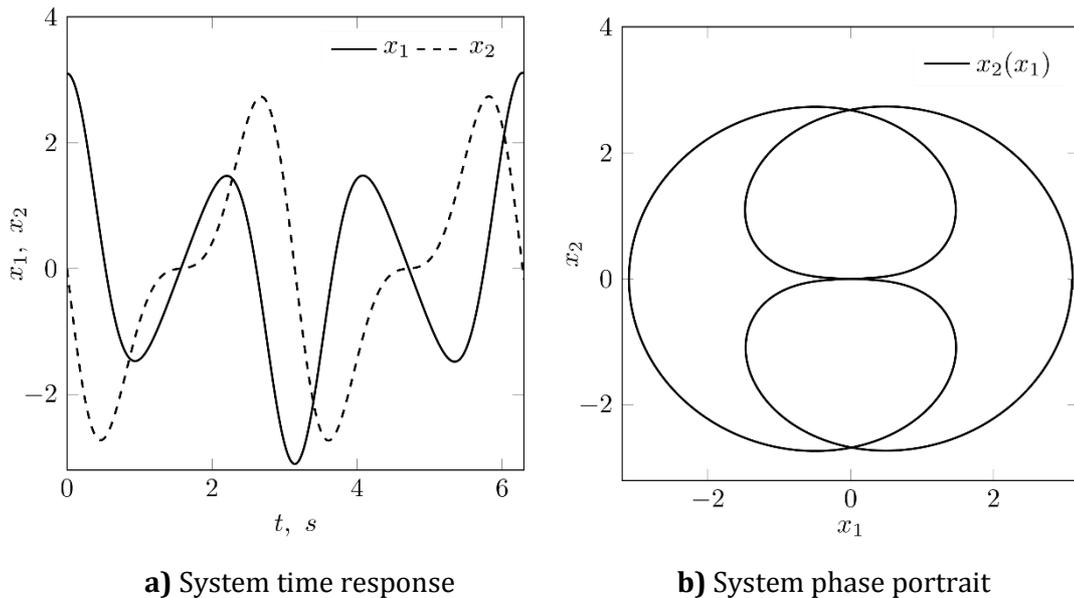
**Figure 3:** Output variables of dynamical system (1) and (2) with initial condition  $y_1(0)=\pi$ .
