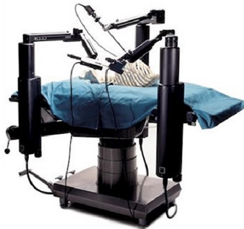
Figure 2. ZEUS robotic system; first robotic system to combine instrument and camera control.
