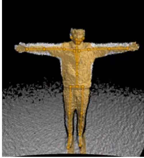
Figure 2: measurement records the three-dimensional joint coordinates [9]
