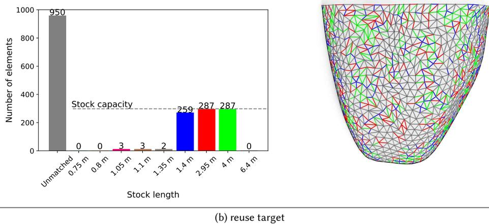
**Figure 3:** Results of our method on a sample freeform shape. (a) Left: the shape provided as input and the multi-target optimized output. Middle: the deformation of the structural nodes under the action of Service Load. Right: the strain energy for each beam. (b) Left: a bar diagram showing the assignment of beams to the input stock. Right: the beam assignment shown through colored edges on the output shape.
