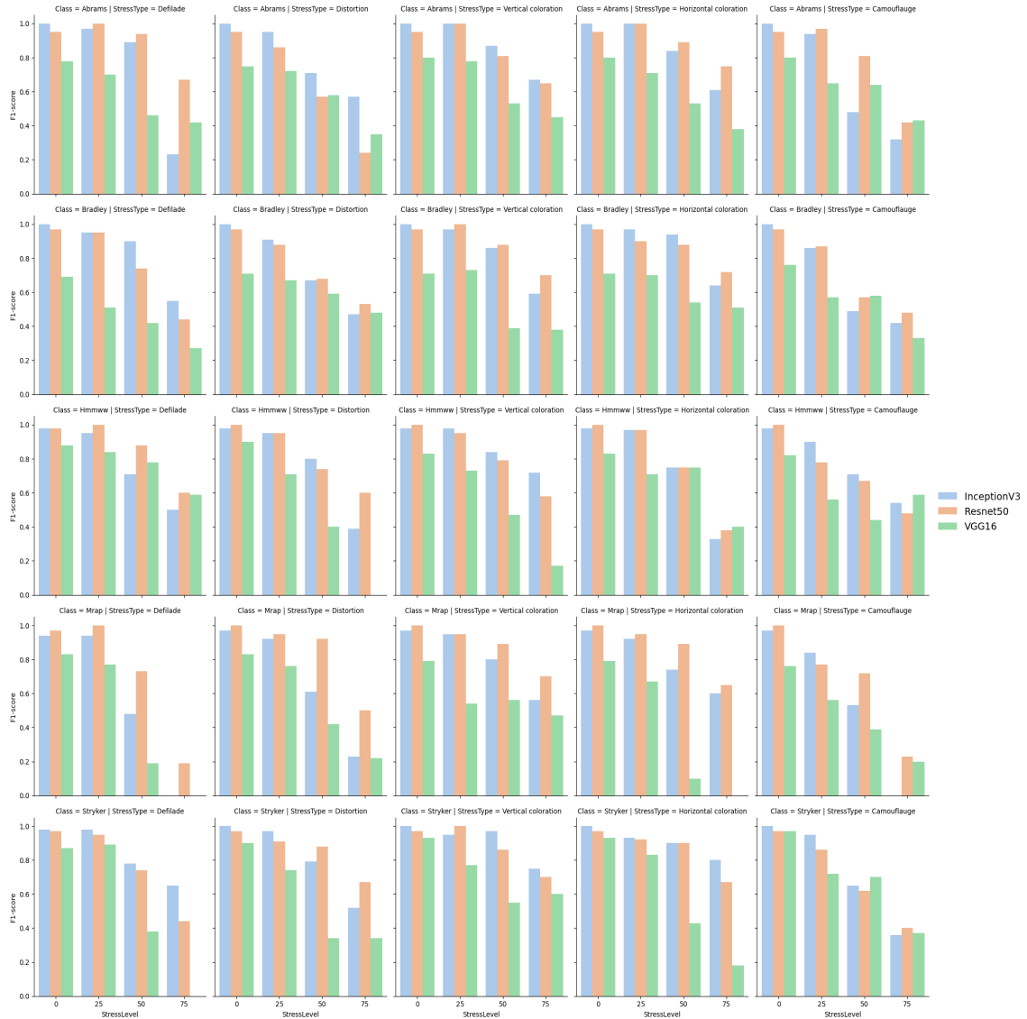
Figure 4: F1-score comparison of the CoNNTText models with different base CNNs (Inception-V3, Resnet-50 and VGG-16). The top row to bottom row represents target classes: Abrams, Bradley, HMMWW, MRAP, and Stryker, respectively. The left column to right column represents stressor types: Defilade, Distortion, Vertical Coloration, Horizontal Coloration, and Camouflage, respectively. Within each bar chart: x -axis represents the stress levels - 0%, 25%, 50%, and 75%, respectively; y -axis represents the F1-score. Blue bar: Inception-V3, Orange bar: Resnet50, Green Bar: VGG16.
