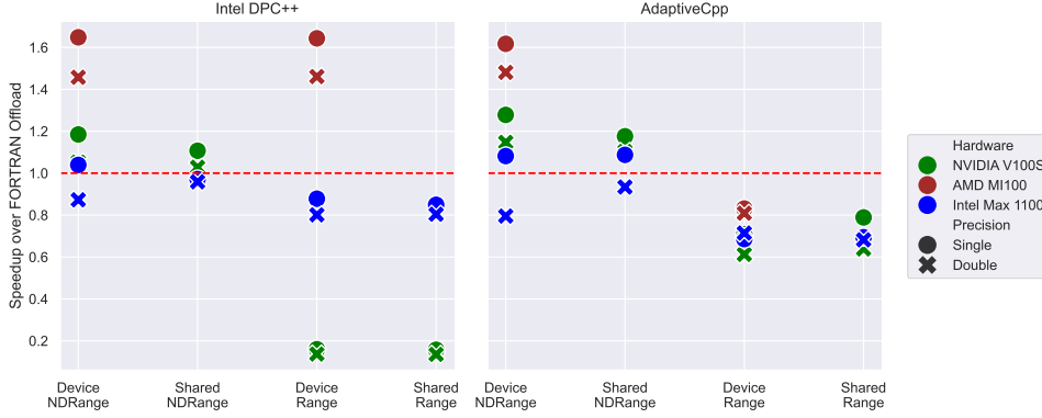
Figure 4: SYCL speedup over FORTRAN offload parallelism model by varying kernel and allocation type with column-major layout and in-order queues, on Lid-Driven Cavity
