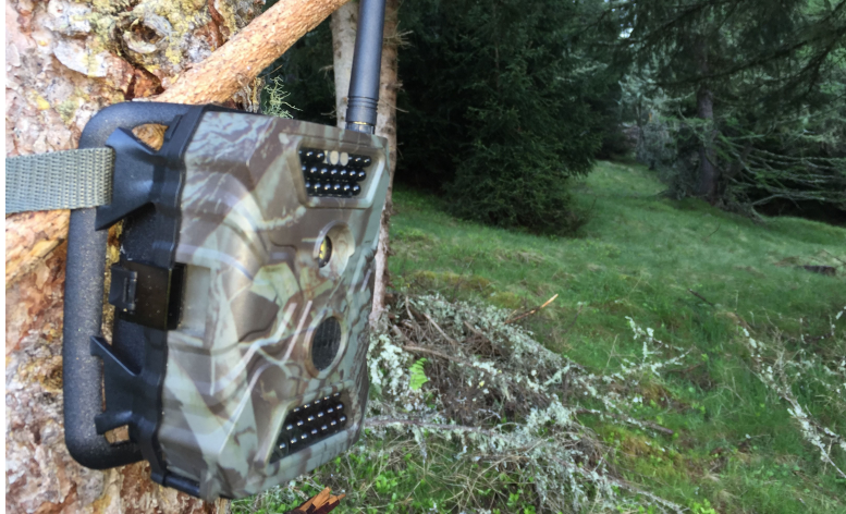
Figure 1: Exemplary trail camera with a SIM card for near real-time data transmission and an infrared flash for night recordings, mounted on a tree to monitor forest activity.
