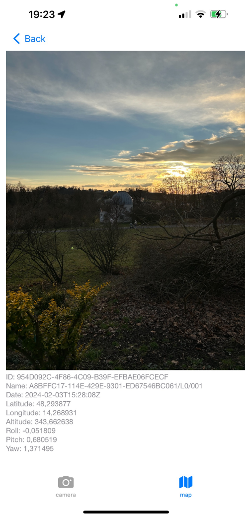
(b) The captured image with the device Euler angles and the GNSS data when the image was taken
