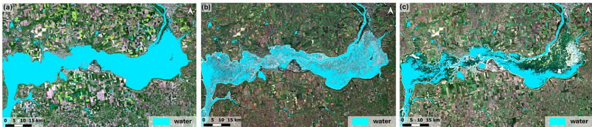
Figure 6: Multi-temporal surface water masks generated using the information tools proposed in this study: (a) before Kakhovka HPP dam collapse on 3 and 6 May 2023. Base image: Sentinel-2 Natural Colour acquired on 06 May 2023; (b) shortly after Kakhovka HPP dam collapse on 20 June 2023. Base image: Sentinel-2 Natural Colour from 20 June 2023; (c) one year after Kakhovka HPP dam collapse on 21 and 25 May 2024. Base image: Sentinel-2 Natural Colour from 25 May 2024.
