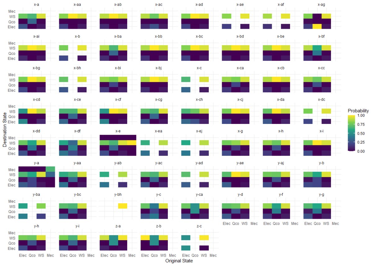
Figure 6: Transition matrices of types of uncontrolled losses per well. The rows represent the destination states and the columns represent the states of origin. Observe that the most probable transitions ( Probability \approx 1 ) occur from any state to a "WS" state ("WS" rows in the matrices). Transitions to "Mechanical" failures are less common (no data in "Mech" rows).
