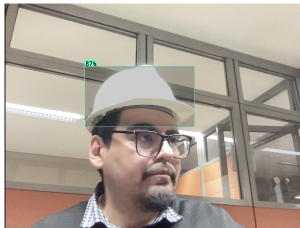
Figure 2: Successful Helmet Detection Highlighting Worker Compliance.
