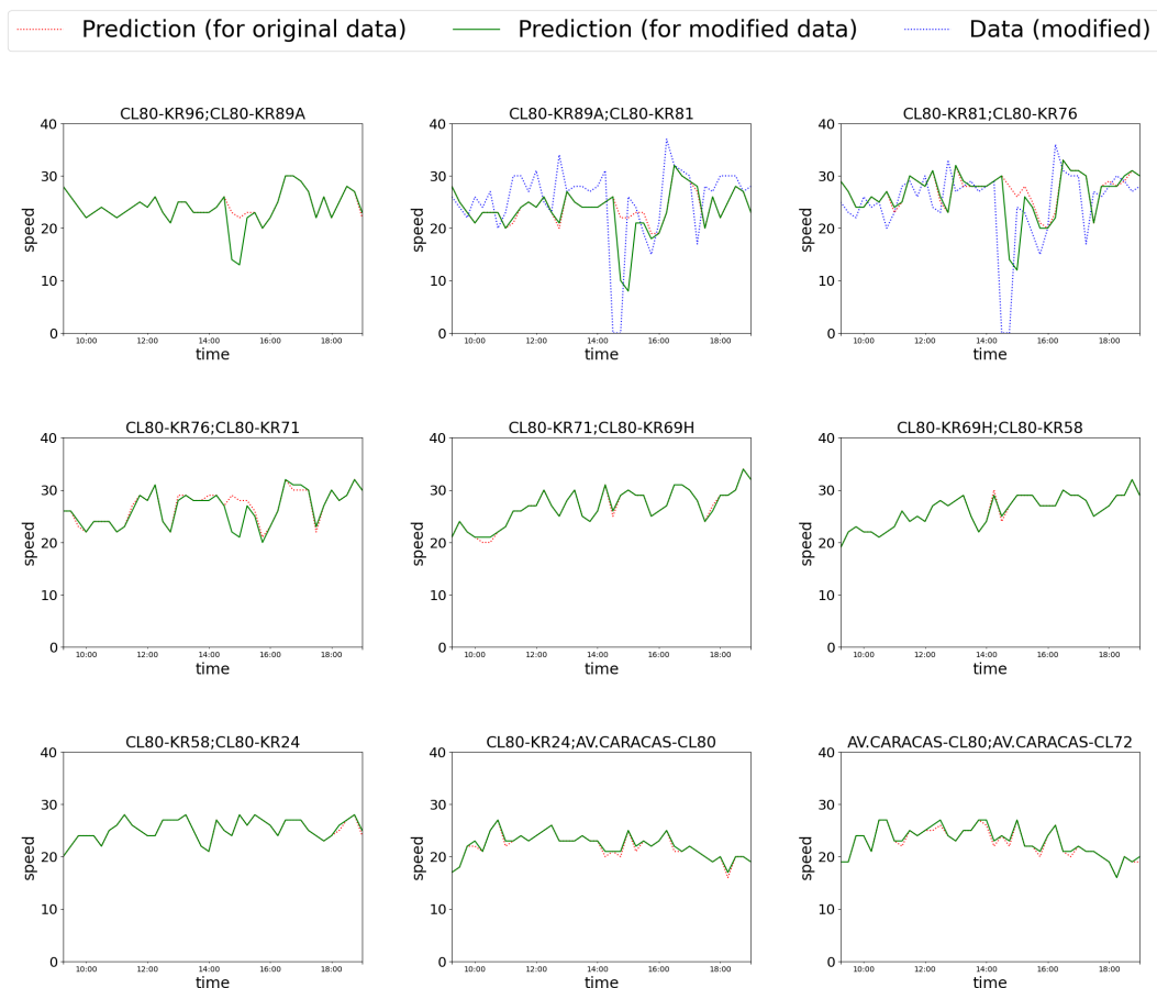
Figure 9: Simulation of traffic speeds from the A3T-GCN model in nodes along Calle 80 and Av. Caracas in response to traffic congestion in two nodes in Calle 80.
