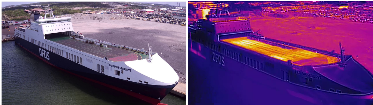
Figure 1: Visual and thermal image of DFDS Petunia Seaways by the UAS prototype (height cropped). Bunker tank visible on left end of thermal image.
