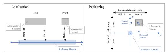
Figure 2: The relationships between infrastructure element and reference element
