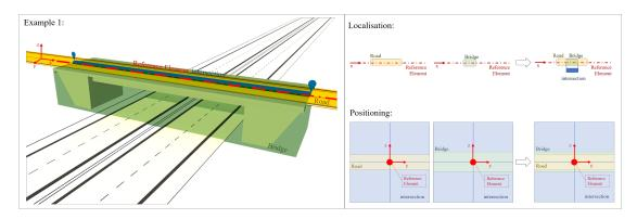
Figure 3: Example 1: A road lies partly on a bridge or a bridge lies on a road
