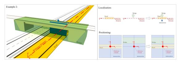
Figure 4: Example 2: A road underpasses a bridge or a bridge overpasses a road
