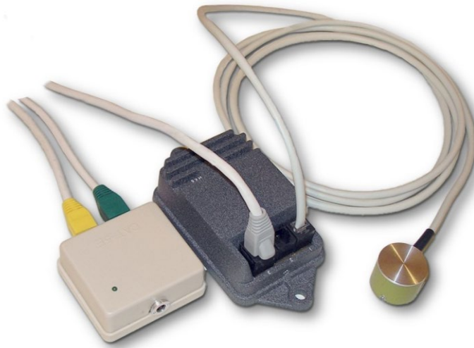
Figure 5: Appearance of the vibration measurement channel
