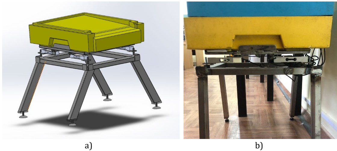
Figure 1: Hive stand with measuring platform and hive bottom a) 3D model; b) finished product.
